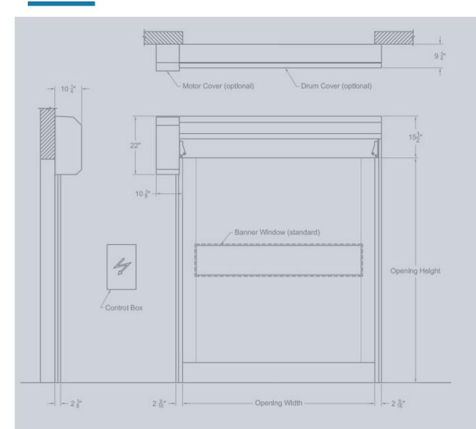
All indicated dimensions are net: the space necessary for mounting and maintenance has to be provided. REMARK: based on the risk analysis of the environment, extra push buttons, detectors and covers might be required.
